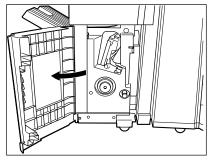
Turn the right-hand knob ① anticlockwise. Then push the left-hand knob ② and turn it clockwise.
